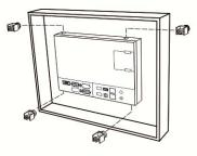
Step 4: For heat dissipation, please keep a minimum clearance of 60 mm on the rear of the HMI.
